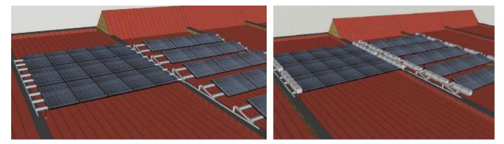
When placed this way, the small beams holding the panels are held down by either brackets attached to the roof surface (as in the illustration on the left) or by ballast at the ends, as in the illustration to the right.
